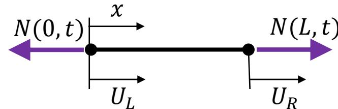
$$\int_0^L \sigma(x, t)A v'(x, t) dx = N(L, t) v(L) - N(0, t) v(0) \quad \dots \text{weak form}$$
