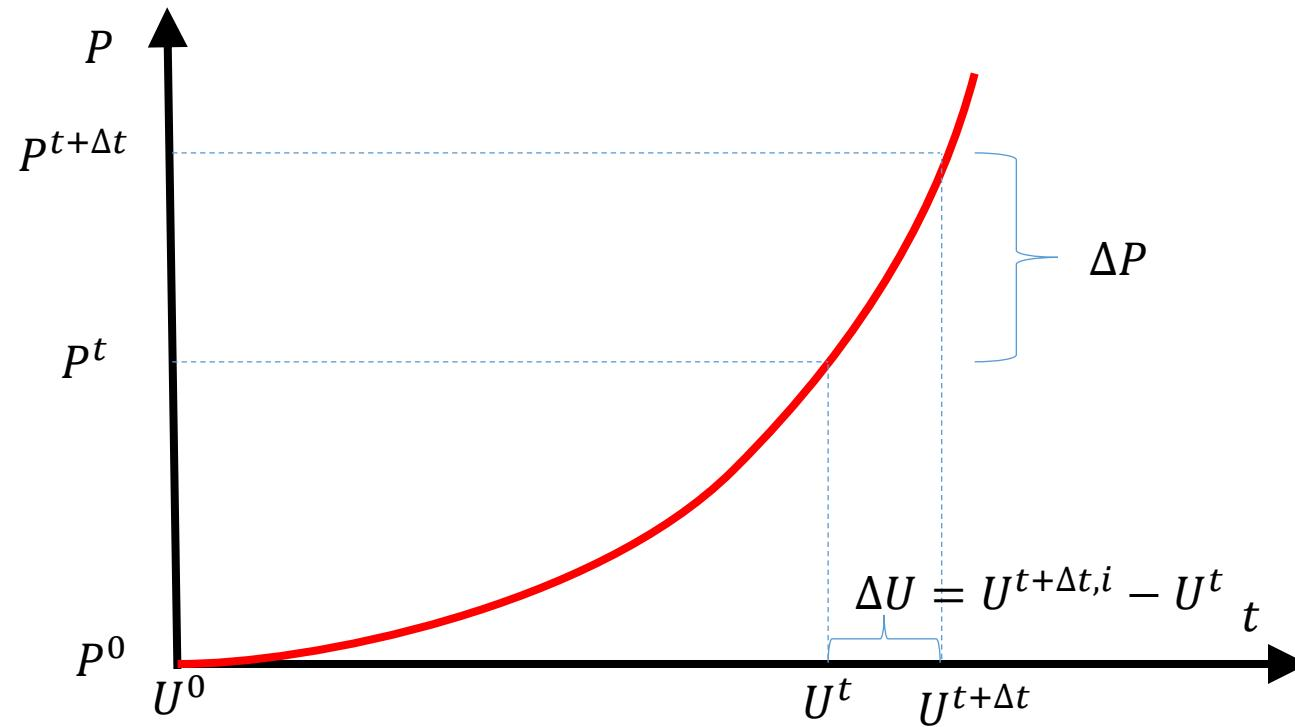
$$\mathbf{F}_{\text{int}}^t(\mathbf{U}^t) - \mathbf{F}_{\text{ext}}^t = \mathbf{0} \quad \dots \text{fulfilled}$$
