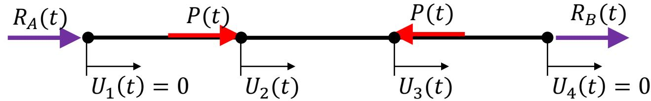
$$\begin{Bmatrix} -\sigma_1(t)A \\ \sigma_1(t)A - \sigma_2(t)A \\ \sigma_2(t)A - \sigma_3(t)A \\ \sigma_3(t)A \end{Bmatrix} = \begin{Bmatrix} -R_A(t) \\ P(t) \\ -P(t) \\ R_B(t) \end{Bmatrix}$$
